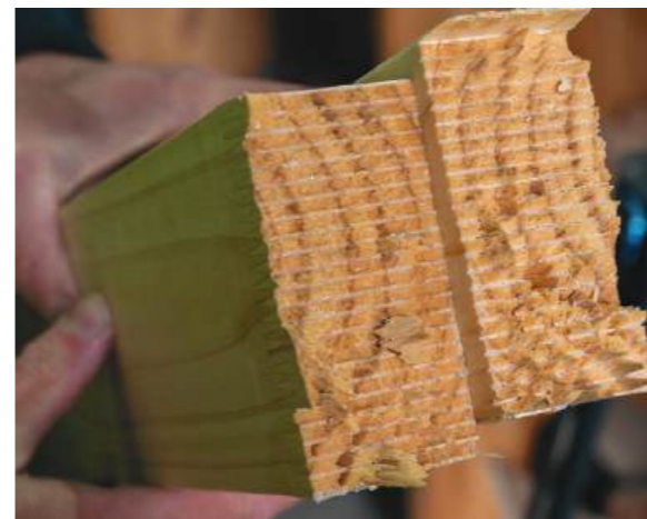
Finger joint strength testing
