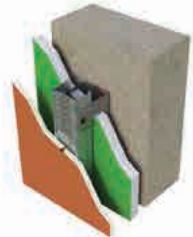
Studco Slimwall system used with foilboard insulation to achieve R1.8 rating.
