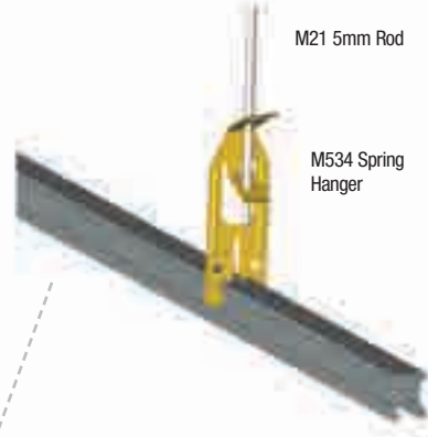
Fig. 5 Top Cross Rail Suspension Clip
