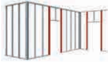
Openings in internal walls
