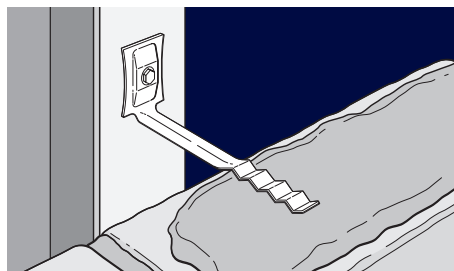
Light Duty Face Fix Sheriff Ties + Hex Screw To Suit .75mm Thick Steel Frame
